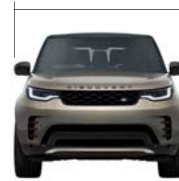
Front wheel track Air suspension 1.692,4mm
